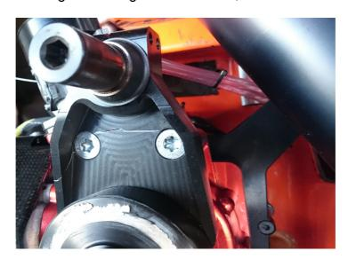
In case of a crash and/or prop strike, the bracket could fail istantly and brake appart into 2 pieces or brake partly as shown. In case of continuous and extensive vibrations due to propeller imbalance the damge can occure in steps where a crack starts to appear between the upper M8 bolts and in consequence continuing to brake the left and right reinforcement walls.
